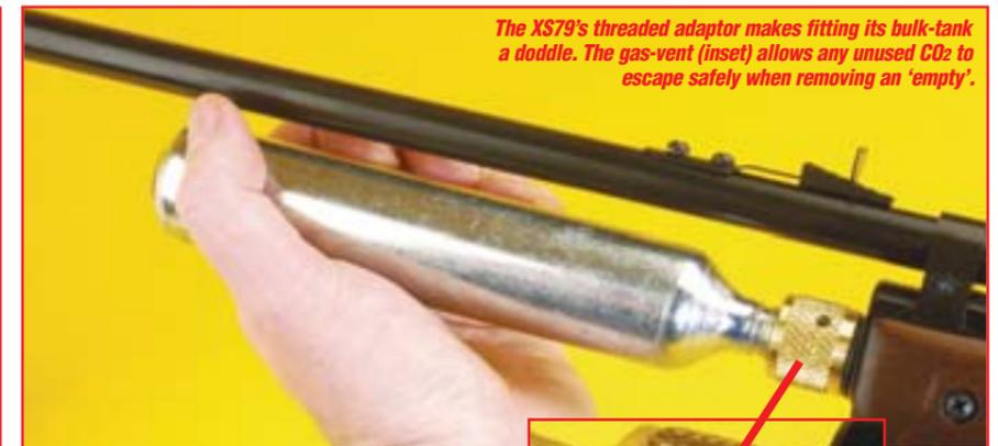
**The XS79's threaded adaptor makes fitting its bulk-tank a doddle. The gas-vent (inset) allows any unused CO2 to escape safely when removing an 'empty'.**
