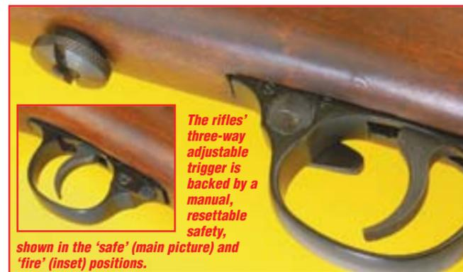
**The rifles' three-way adjustable trigger is backed by a manual, resettable safety, shown in the 'safe' (main picture) and 'fire' (inset) positions.**
