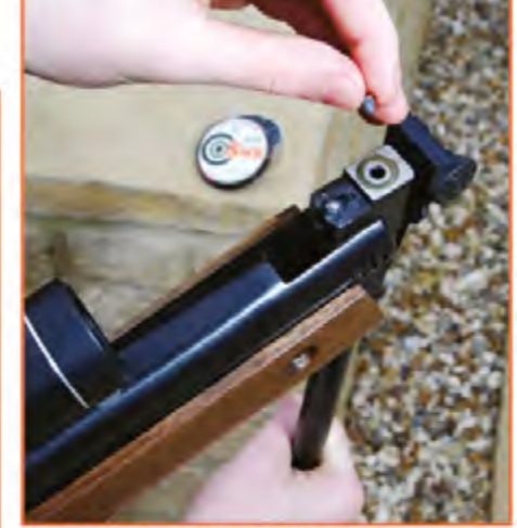
Loading the break-barrel action. Thanks to its modest power, cocking the Super Grade 15 is also 'teenage-friendly'.
