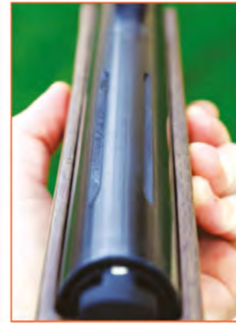
The Super Grade's receiver is grooved to take a scope (above), and has an automatic, resettable safety catch (below) at the end.
