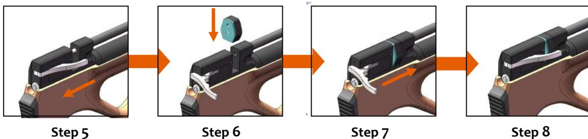
FIG 6 LOADING PROCEDURES
